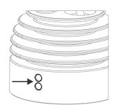
NOTE: THERE ARE TWO FIXING HOLES ON THE LED ENGINE.
