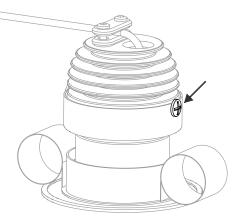
ONCE ASSEMBLED USE THE TWO PHILLIPS SCREWS PROVIDED ON THE LED ENGINE TO FIX INTO PLACE INSTALL.
